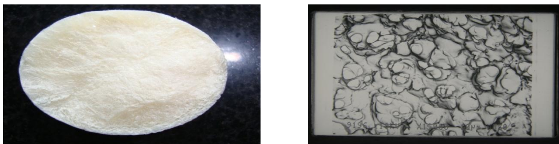
Fig.1. Characterization of chitosan porous matrix scaffold formulation. Photographs of top and SEM views of scaffold formulation respectively.
