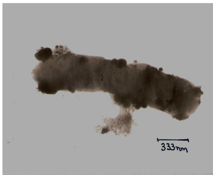
Figure 3: Transmission electron micrograph of silver nanoparticles embedded on Lactobacillus sps VRS-2
