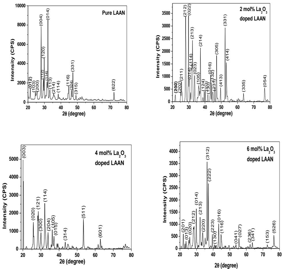
Fig. 3. The Powder X-ray diffraction patterns of pure and lanthanum oxides doped LAAN crystals
