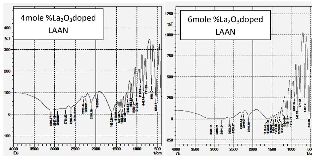
Fig. 4. FT-IR spectrum of a pure and lanthanum oxides doped LAAN crystals
