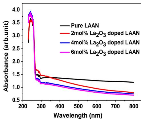
Fig.7. The absorption spectrums of pure and lanthanum oxides doped LAAN crystals
