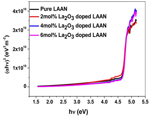
**Fig9.**  $(\alpha h\nu)^2$  vs photon energy ( $h\nu$ ) plot of pure and lanthanum oxides doped LAAN crystals
