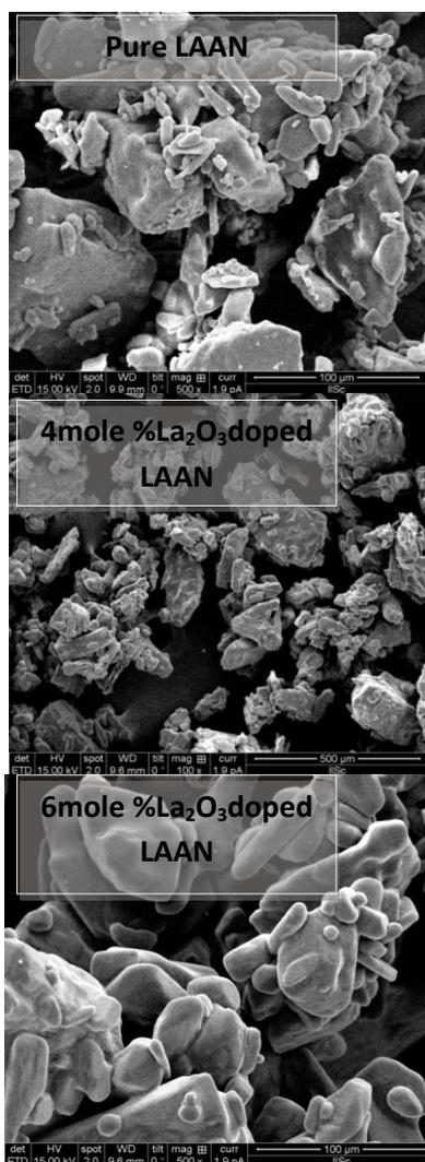
Fig. 5 . SEM images of pure and lanthanum oxides doped LAAN crystals
