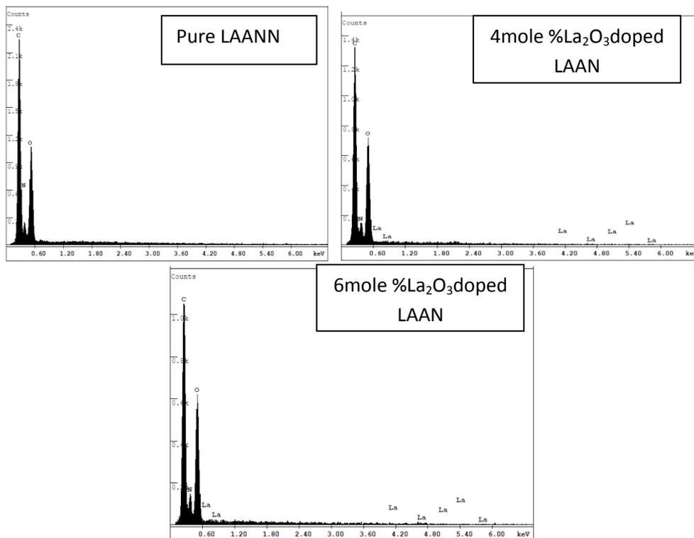
Fig. 6. EDX of pure and lanthanum oxides doped LAAN crystals
