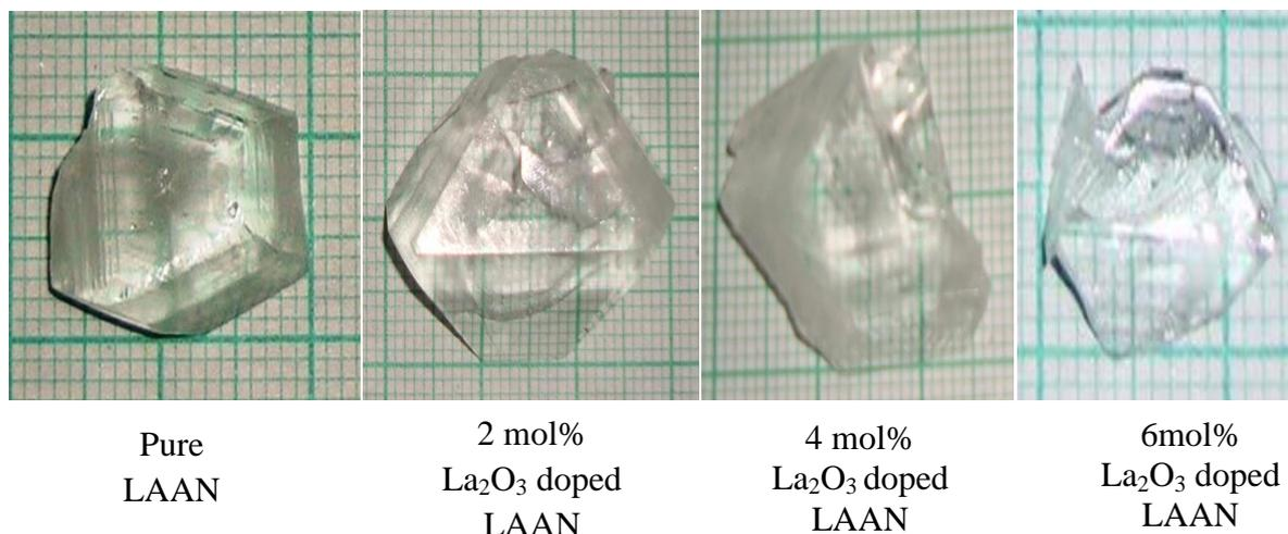
Fig.2. Photographs of the as grown pure and lanthanum oxides doped LAAN crystals
