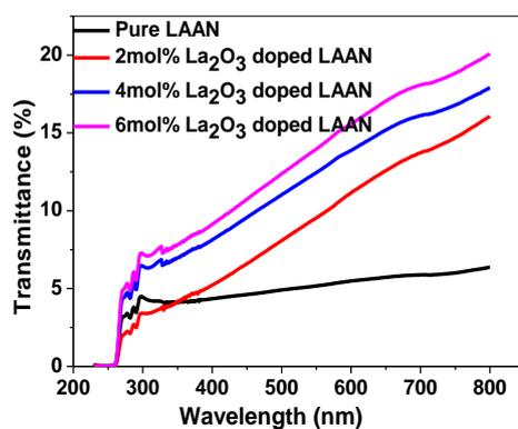
Fig 8. The transmission spectrums of pure and lanthanum oxides doped LAAN crystals
