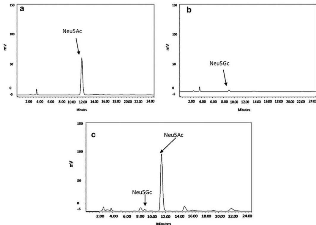
**Fig 1: Chromatogram of the Neu5Ac–DMB standard 150 ng (a), Neu5Gc–DMB standard 5 ng (b), and IF A1 sample (c).**
